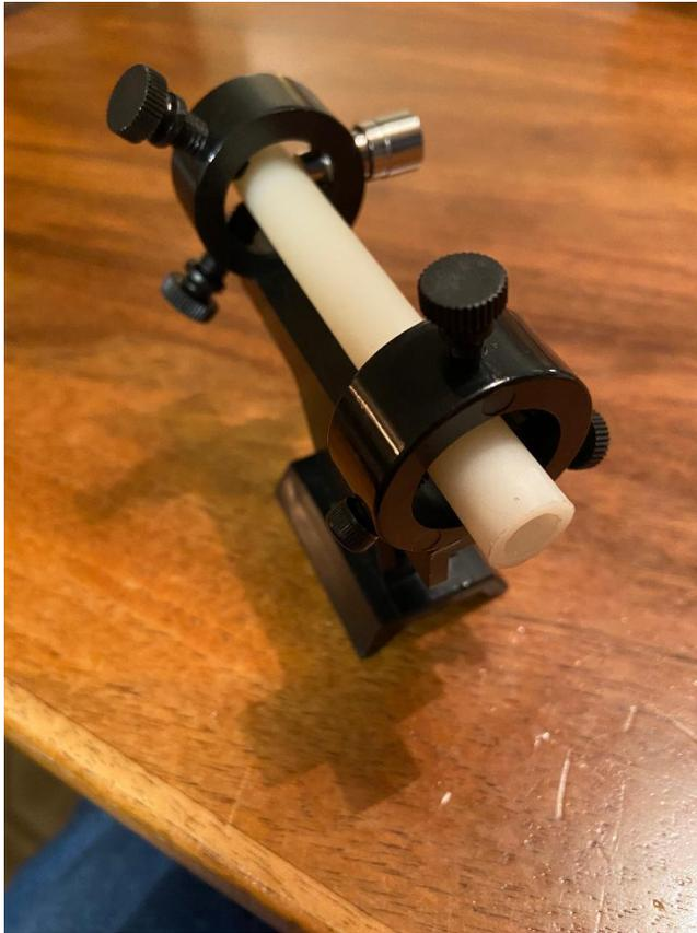
The plastic pipe is 4 inches long and has a hole through it  $\frac{1}{4}$  inch in diameter. This hasn't been tested out yet but we believe it has a field of view slightly larger than the full moon. There is no cross hair so there may be some concern with parallax. The mount would cost less than \$20.
