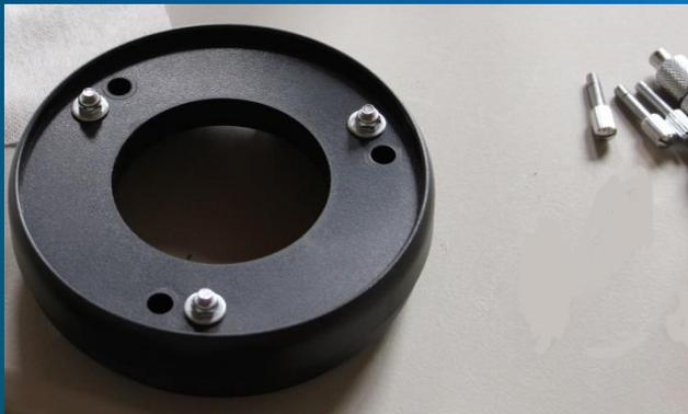
3. Install washers and locknuts
