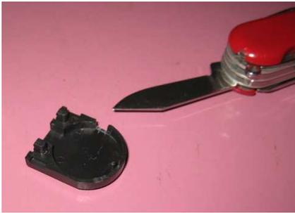
Next, we cut a notch in the left side of the battery cover. This keeps the wires away from the sharp edges of the battery clip. A dremmel tool works very well for creating the notch.
