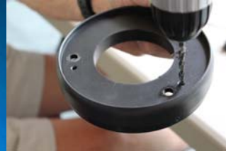
2. Drill out small holes to 15/64
