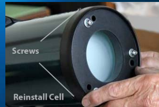
4. Reinstall mirror cell
